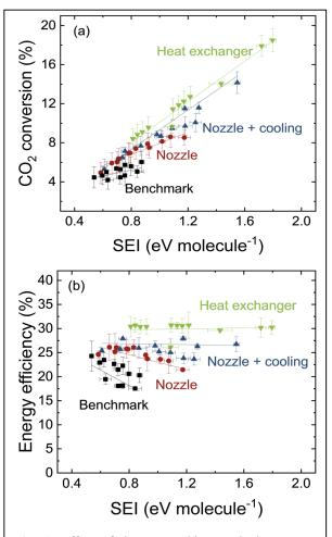
Fig. 1. Effect of three quenching methods on  $CO_2$  conversion (a) and energy efficiency (b), compared to the benchmark, as a function of SEI.
